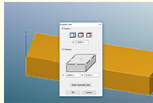
The zero should usually be at the bottom left corner at the top of the work stock.
