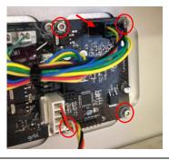
**Step 5:** Remove motor driver by sliding it away to the right from the second connector.
