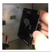
**Step 6:** Remove thermal compound with dry paper towel (optional rubber alcohol with Q-tip).
