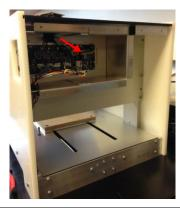
**Step 4:** Remove motor driver hardware (four 3M screws) and connector from top of PCB board.
