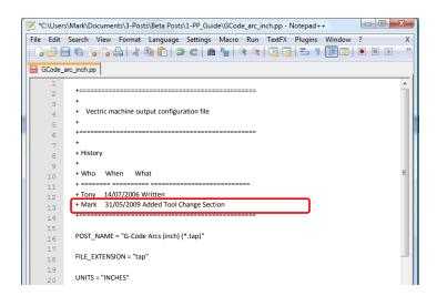
Next edit the POST\_NAME to reflect that this post processor outputs automatic tool change (ATC) commands, the new post will be displayed as "G-Code ATC Arcs (inch)(\*.tap)" in the list of post processors.
