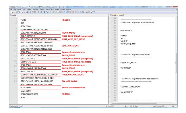
The post processor configuration files are located in the "PostP" folder for the application. The post processor configuration files have a ".PP" file extension.
