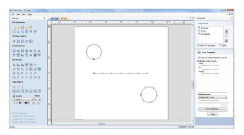
Save a toolpath using your base post processor and take a look at it using your favourite text editor. Below is an example of the test file posted using the "G-Code Arcs (inch) (\*.tap)" post processor The example below is displayed using the popular Notepad ++ editor.
