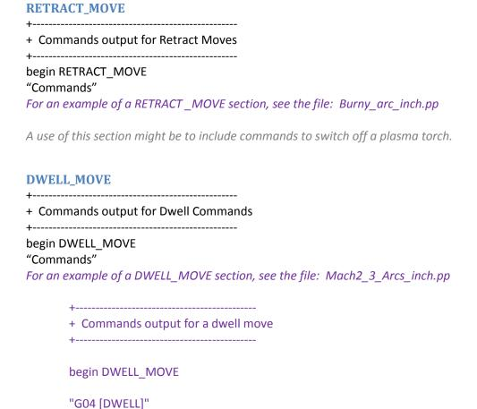
This command was introduced for VCarve Pro 7.5 and Aspire 4.5 and later. It is used with a drilling toolpath, when a Dwell time has been specified in the program. If this section is not defined any dwell commands are ignored, but the rest of the drilling toolpath will be output as normal. The DWELL variable is documented in the Variables section.
