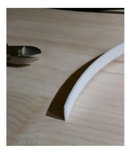
Buying several meters of steel-core belts is cheap, will serve as a provision in case the original belts snap, and replacing the belts is very easy (since it does not involve disassembling anything else other than the belt tensioners) so that upgrade is a no brainer if you feel you can benefit from the increased robustness, and possibly from the ability to push the max speed and acceleration beyond the default settings:
