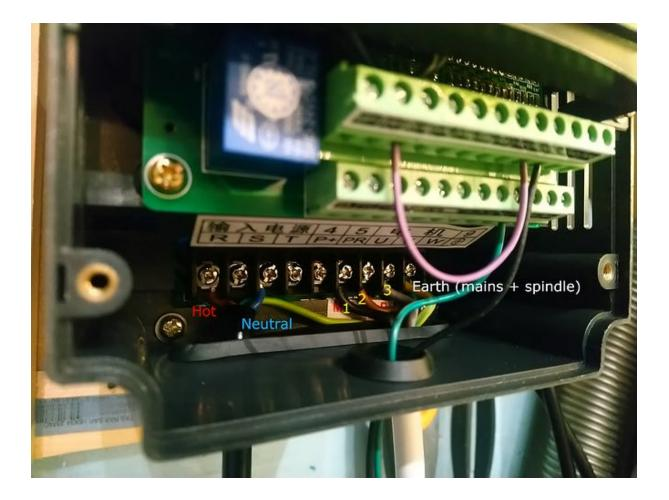
Make sure the spindle's **ground/earth pin** is actually connected inside the spindle to the body:
