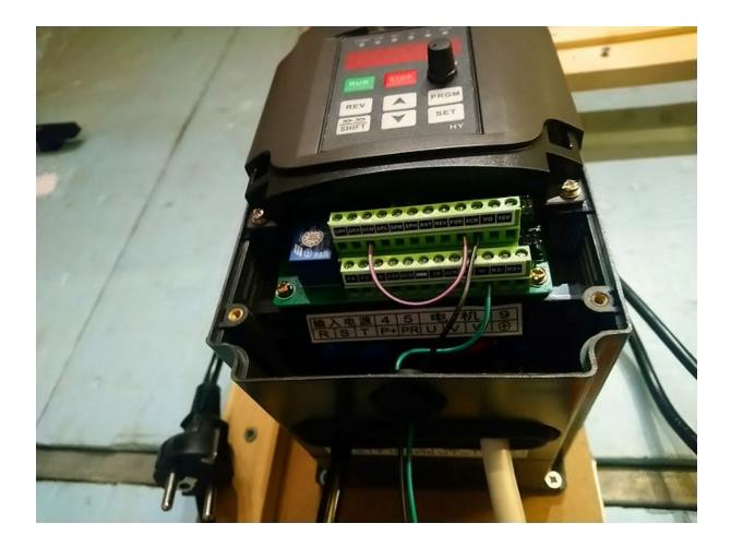
Beyond that it's just a matter of connecting mains, and the four wires to the spindle (1,2,3 and Earth, also called U,V,W and Earth):
