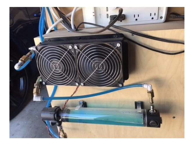
A section of the cooling loop should have fans, to keep the coolant temperature down.
