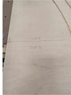
I loaded the file “rocker\_tile1” into Carbide Motion and started the job. The tile 1 completed. The cutting was 24.25” long because I had set for a .25” vertical overlap. The tile was 24” long but the vertical overlap was added.
