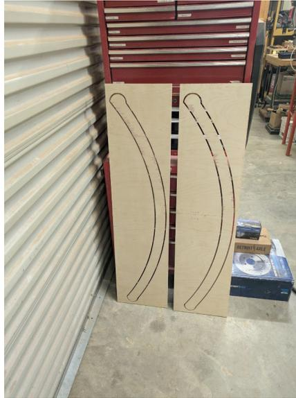
This was my first tiling job and it turned out well. If these prototypes work I will cut the actual rockers out of 2" oak. I will use a different bit because the #201 does not have the capacity to cut 2" I have a Melin bit that will cut through 2" material.
