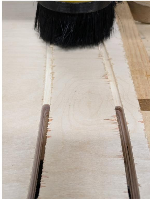
You can see that towards the top of tile 1 the chipout increases as the grain of the veneer was almost 90 degrees to the bit and increases in tile 2.
