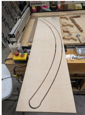
The router cut .25” back inside the previously cut tile 1. This is the vertical overlap set in the tool path. You can decide how much overlap you want in the tool path tiling setup.
