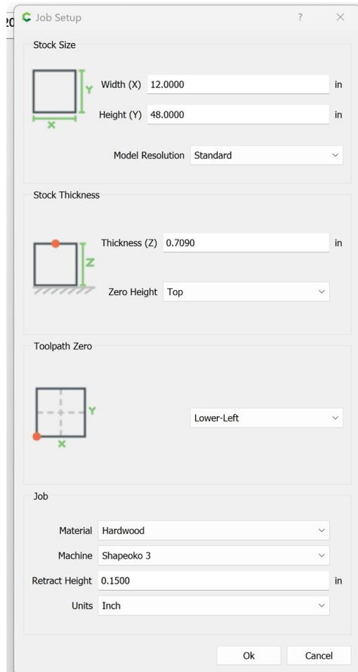
I had bought some birch plywood that was made in Indonesia that only measures .7". I used my new Milescraft Track Saw Guide to cut the plywood up into 12" strips across the 48" width. I have a large tablesaw but find it hard to handle full sheets of plywood by myself and this track saw worked perfectly. Under the material is a piece of 1" 4'x8' foam. Dont cut through your foam.
