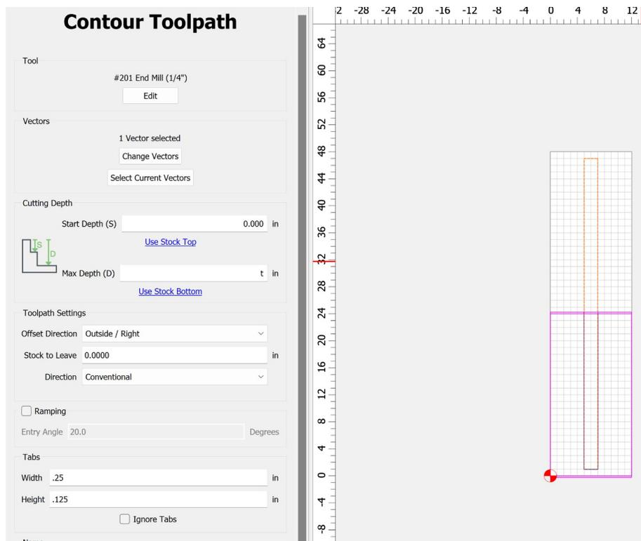
After creating the tool path I saved the file as "rocker\_tile1.c2d". You have to save each tile as a separate file. Once the first tile runs the machine will stop and you move your material and load the second tile and so on and so on as many tiles as you make. In my case I have 2 tiles so I have 2 files "rocker\_tile1.c2d" and "rocker\_tile2.c2d".
