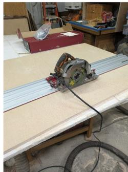
The 48” length is longer than my SO3 XXL so I made a tiling job. I highlighted my rocker and went to tool paths and selected an outside contour with the #201 upcut bit. I checked the “Toolpath Tiling (Pro)” box and I believe it defaulted to a 20” tile which would have required 3 tiles on a 48” length material. So I edited that to 24” so I would have 2 tiles and only have to move the material once.
