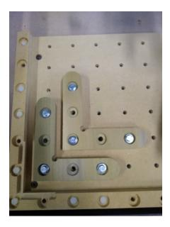
The first consideration is how big your brackets should be. These are 6 inches by 6 inches with 5 holes and a corner relief. Set up a grid pattern that is a multiple of the width of your L brackets and check snap to grid. In this case I set up .25 inch grid pattern.
