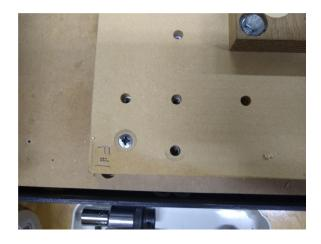
With the 1/4-20 Tee Nuts I use an L bracket and cam clamps to secure projects to the spoilboard. I am using the painters tape and super glue more and more and especially for small projects. I use the L bracket for the initial gluing and then remove it. It is important to replace the L bracket before removing the project because I use the router with a bit in it to initially square the L bracket.
