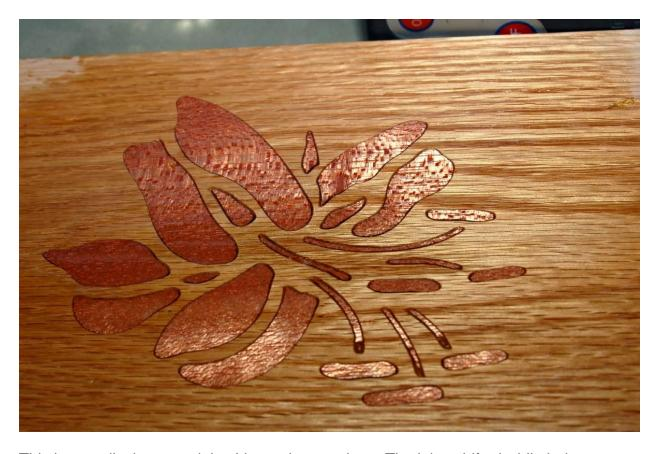
This is actually the worst inlay I have done to date. The inlay shifted while being cut do to insufficient clamping. Even so, the process is very forgiving.
