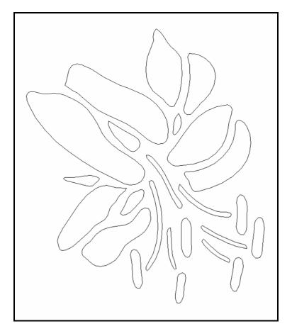
Summary of this section – The pocket artwork must be flipped left to right to create the inlay, A "hog out area" is defined around the inlay, and finally, the inlay cut file is computed with a 0.1" start depth and a 0.2" flat depth.
