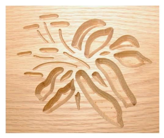
This is the male inlay and backing before the excess wood under the clamps is cut off
