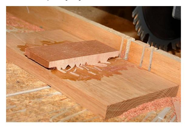
The backing has been cut off and it is ready for sanding. (The clear shiny stuff is superglue.)
