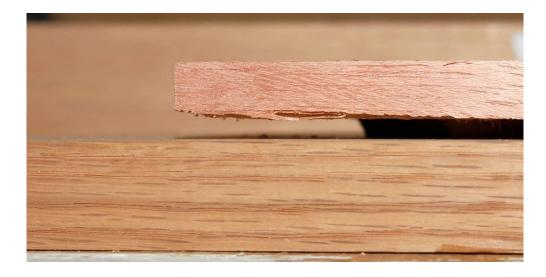
I usually copy the position of the inlay onto the pocket piece with a pencil. This makes it much easier to reposition the inlay after glue has been applied.
