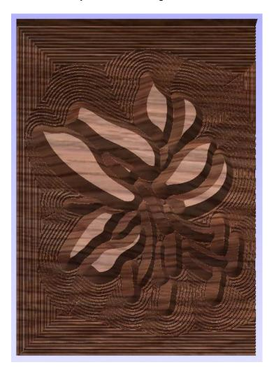
Even though it looks all wrong, it does fit correctly. The ridges are an artifact of the 13% stepover which was used to reduce hog out cut time. They are in the inlay backing and will be removed when the backing is removed. If one decided to use an end mill for hogging, the ridges will not appear.
