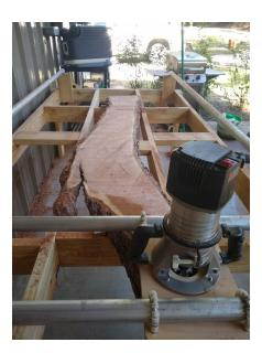
The slab was cut to rough size and marked with white pencil to trim on the bandsaw.
