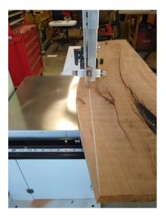
This is resawing the slabs after cutting them straight on one edge.
