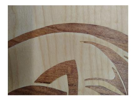
Got the table top female socket carved today. Talked to Grandson and I will make a maple inlay to go into the table top. I will still fill cracks and defects with black epoxy. On the bottom of the top there is some stress cracks that will also need to be filled.
